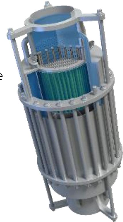
The dual function of fuel supply and heat removal in the MSR limits the power density. Dual Fluid overcomes this limitation.
